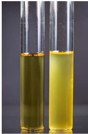
Azide Dextrose Broth; from left: uninoculated tube and tube with Enterococcus faecium .
